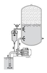
When starting, the pumps creates a suction pressure which also takes the water from ARIAMAT, allowing some more water to come from the vessel. The water through the ARIAMAT venturi sucks air from the upper valve.
