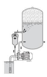
When stopping, there is a back-flow of water from the vessel through the pump, to the ARIAMAT. Air is pushed inside the vessel.
