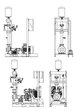
UNI-EN 12845 units for feeding fire-extinguishing systems with 1 N series electric main pump
