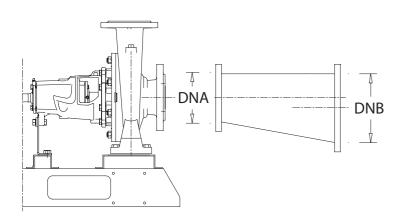
Flanged reductions eccentric to be installed in the suction of main pumps, are complete of 1/4" out point, ball interception valve and vacuum gauge (or gauge on request).
